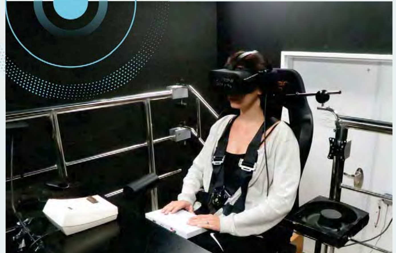
Dr. Zaidel's custom, 3D multi-sensory motion simulator with virtual reality glasses for studying how the brain integrates information from multiple sources.
